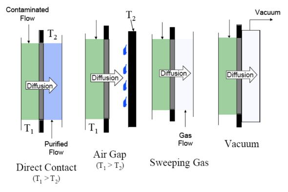
Figure 9: Different membrane distillation process
