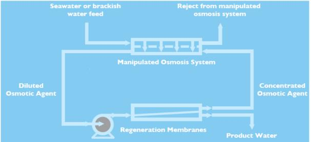
Figure 12: Modern Water's Manipulated Osmosis Desalination Process
