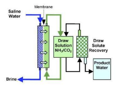
Figure 11: Simplified process schematics of FO
