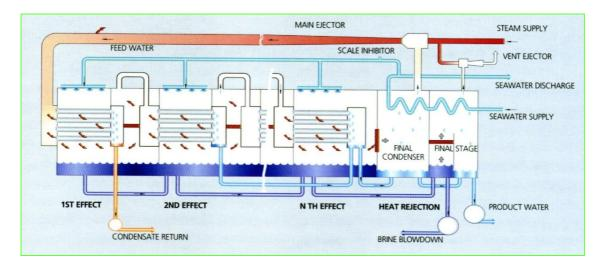
Figure 2: Schematic diagram of a simple MED-TVC unit
