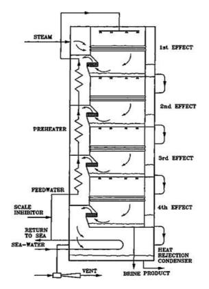
Figure 19: Schematic diagram of the Multiple Effect Stack (MES) flow configuration
