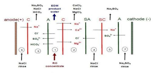
C = ordinary cation exchange membrane A = ordinary anion exchange membrane SC = monovalent selective cation exchange membrane
