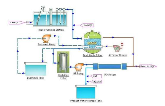
Figure 5: SWRO process schematics
