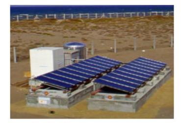
Figure 20: A 1 m3/d multiple effect HDH unit in Oman
