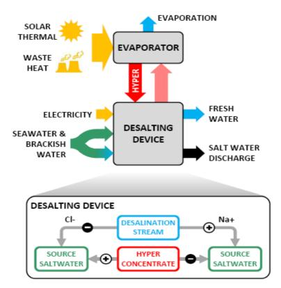
Figure 10: Schematics of Saltworkstechnology [34]
