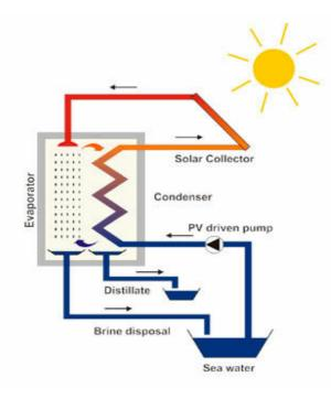
Figure 15: Simplified process schematics of HDH
