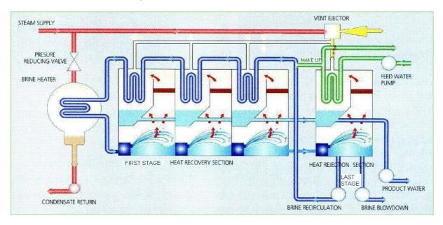
Figure 1: Schematic diagram of a simple MSF Unit
