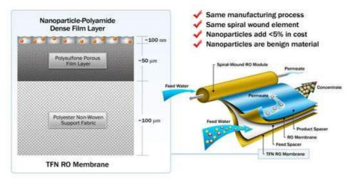
Figure 6: Nano membranes by Nano H<sub>2</sub>O
