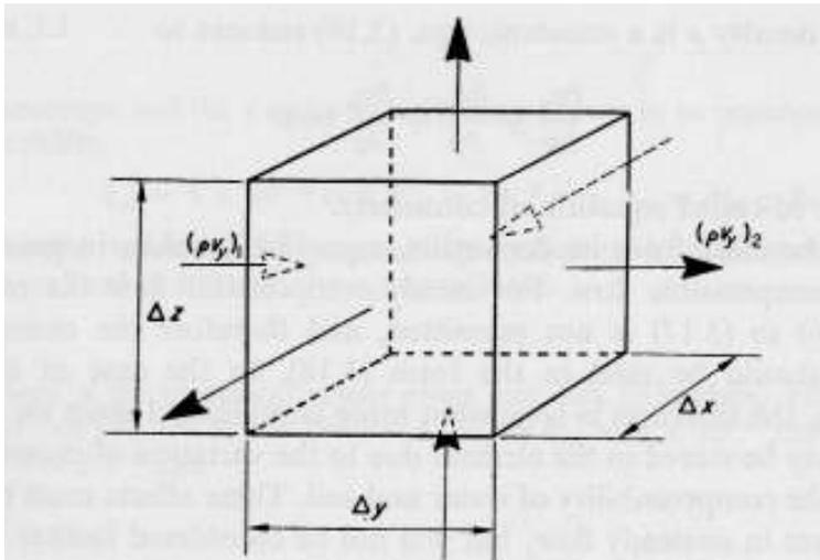
FIG. 3.4 Specific mass discharges into and out of element
