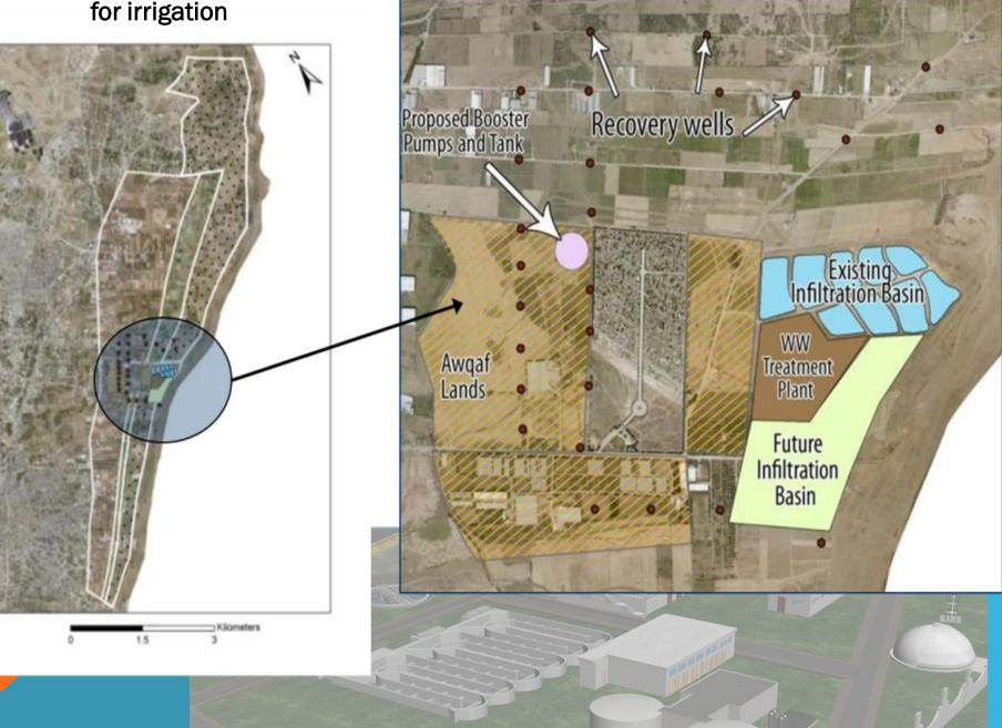
Components of Effluent Recovery and Reuse Scheme includes:
