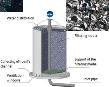
Aerobic process, where the wastewater, after receiving prior treatment (pretreatment and primary treatment), percolates by gravity through a filling material (stones, plastic material), which constitutes the medium on which microorganisms develop and grow, forming a biofilm of variable thickness. The filling material is fixed, inside the reactor, and provides a high specific surface area.
