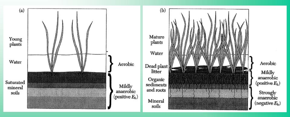
Figure 1.5. Stages in the maturation of constructed wetland soils: (a) newly planted, (b) mature (Kadlec & Knight 1996).
