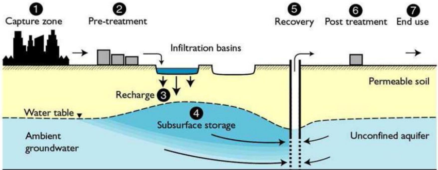
SAT system for pre-treated wastewater, infiltrating through recharge basins into permeable soil (unsaturated zone) and recharging the groundwater aquifer. Source: MIOTLINSKI et al. (2010)
