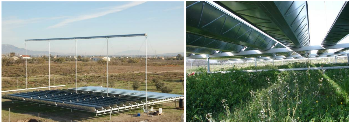
Figure 1-18: Novatec-Biosol linear Fresnel collector prototype at Lorca, Spain
