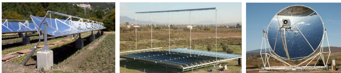
Figure 1-31: Left: Low-temperature parabolic trough for direct steam generation from SOLITEM, center: linear Fresnel from NOVATEC-Biosol, right: Dish-Stirling engine from Schlaich, Bergermann & Partner
