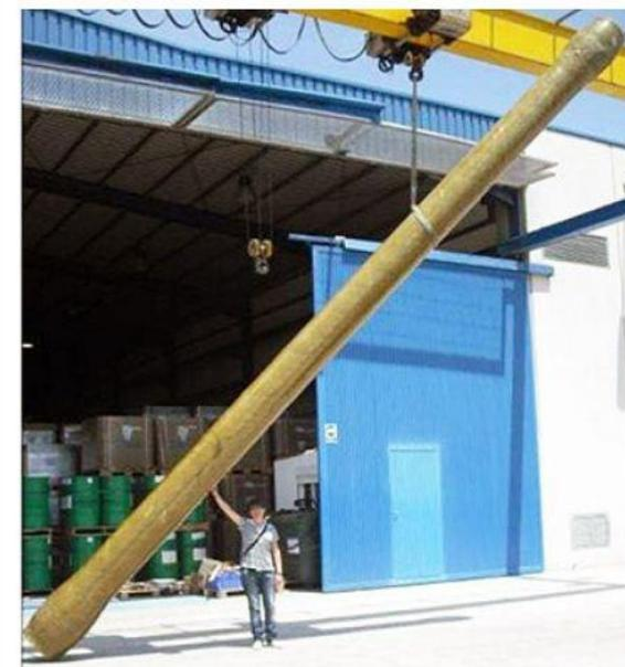
*BEL's 16-inch diameter, 8-element Pressure Vessel*
