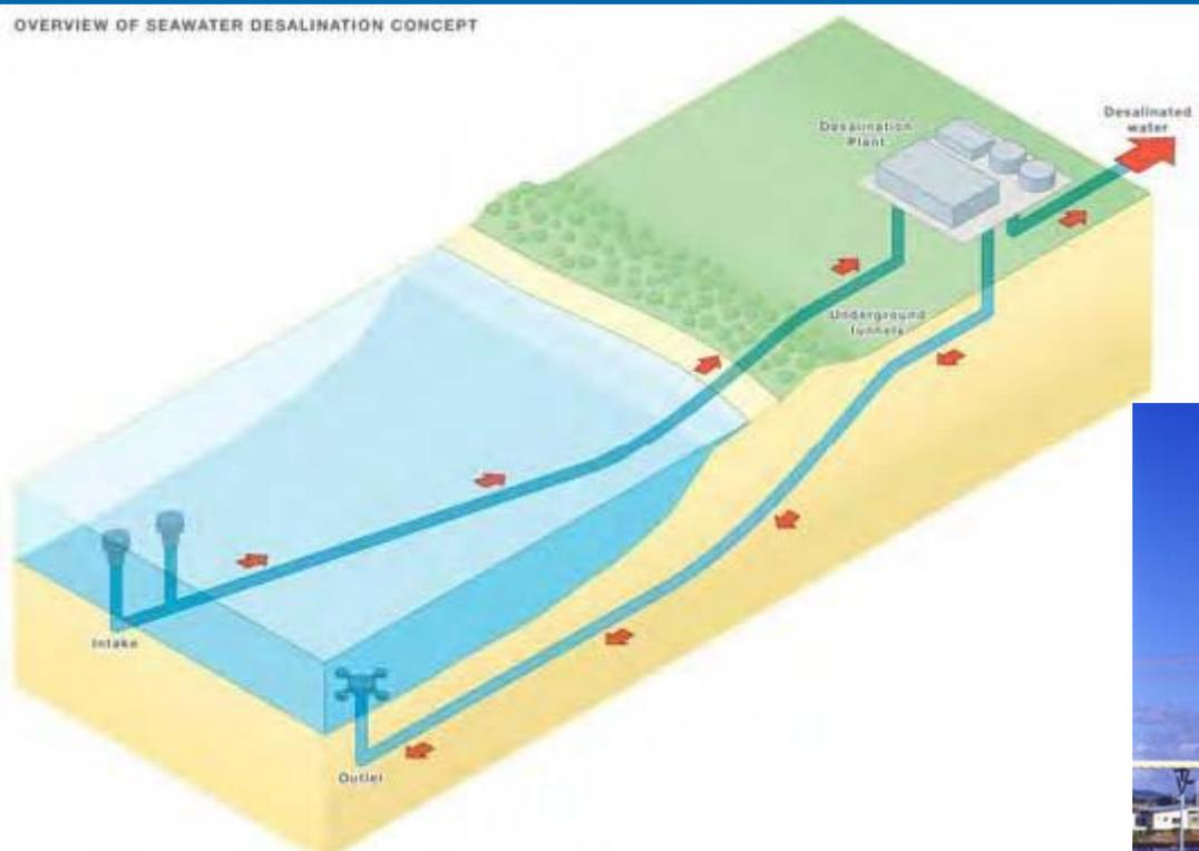
**Off-shore Intake for Sydney Water Desalination Plant, Australia**
