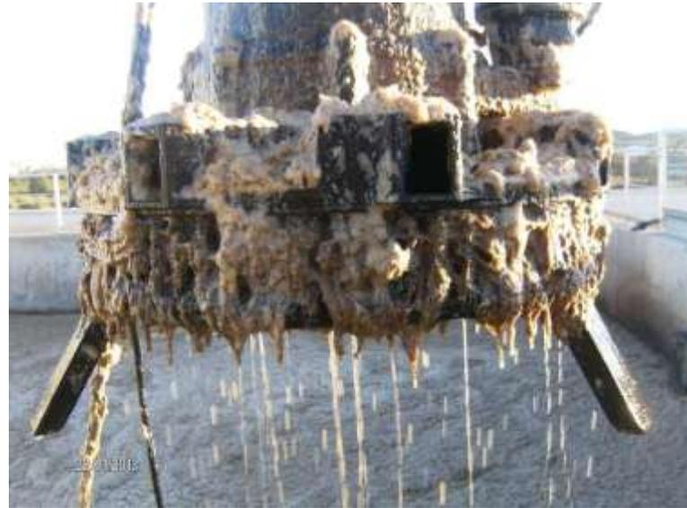
Turbid effluent because of aeration deficit and submersible aerator clogged with fibers.
