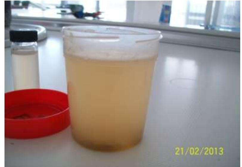
Orange color due to an illegal discharge to a WWTP
