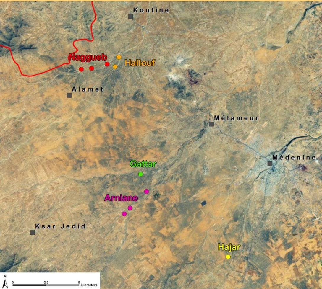
The design of the managed aquifer recharge system consist of 10 **recharge wells**, equipped with recharge chambers, placed in the centre of the wadi upstream of existing gabion check dams which usually retains the flooding water during rainy events. We estimate overall an average of 1.2 Mm<sup>3</sup>/year.
