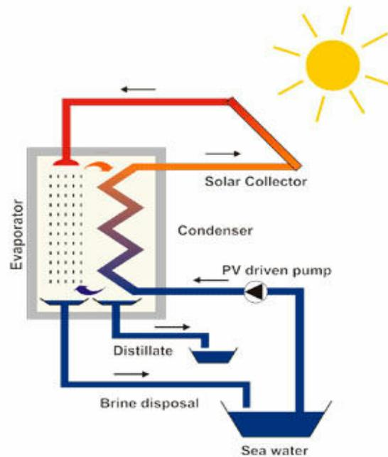
Figure 15: Simplified process schematics of HDH
