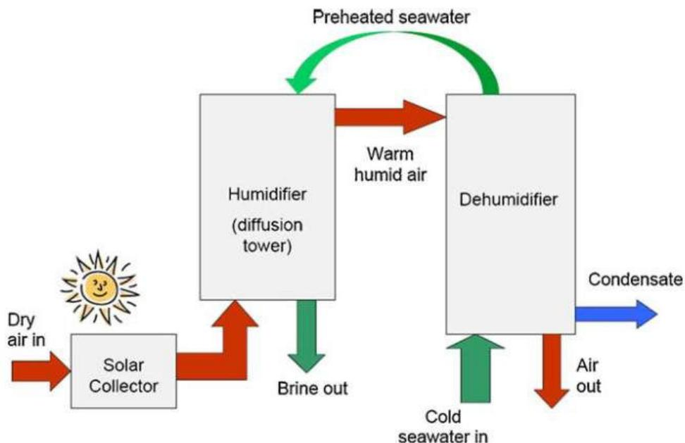
Figure 16: Simplified process schematics of HDH with solar heat transferred by air
