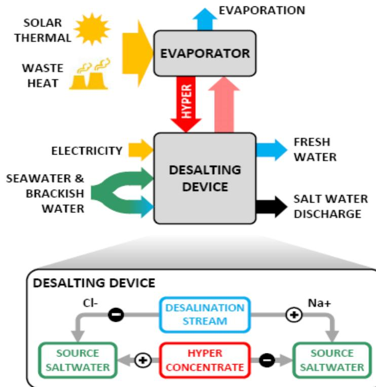
Figure 10: Schematics of Saltworkstechnology [34]
