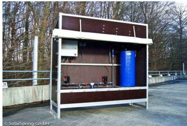
Figure 22: A view from the backside of the Oryx 150 unit. The spiral-wound MD module is the blue vessel on the right.
