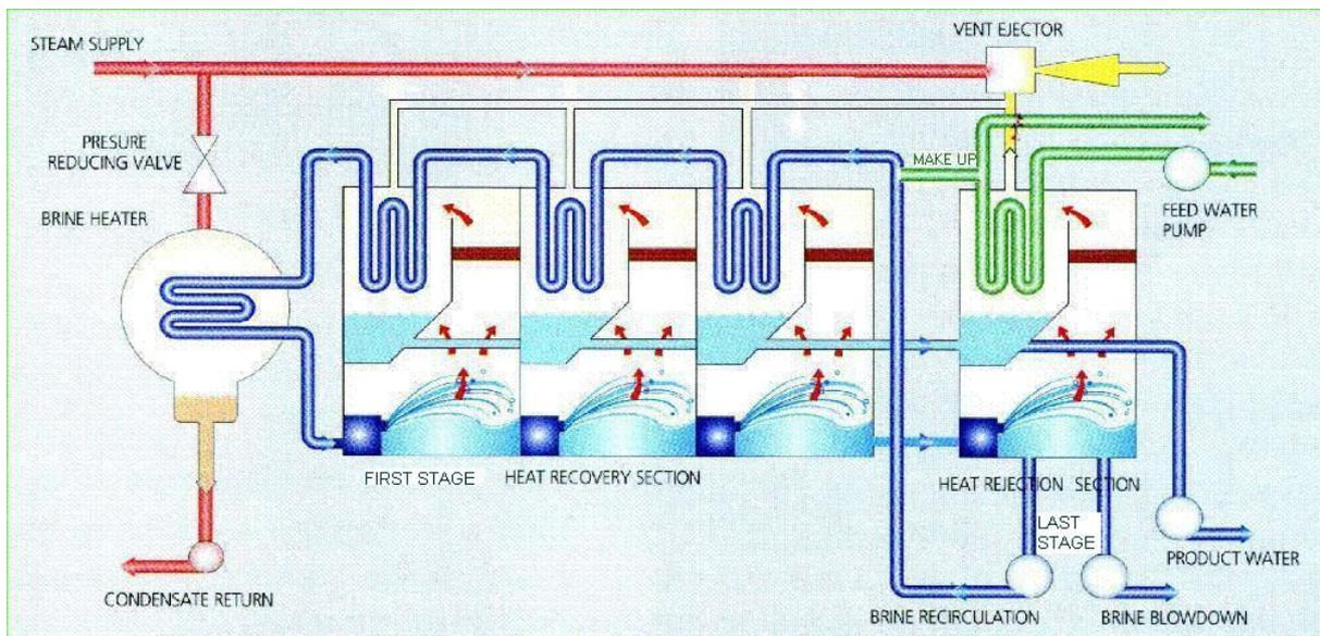
Figure 1: Schematic diagram of a simple MSF Unit
