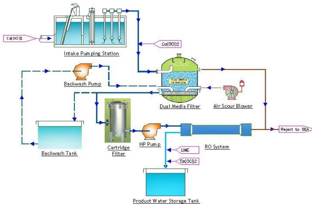
Figure 5: SWRO process schematics
