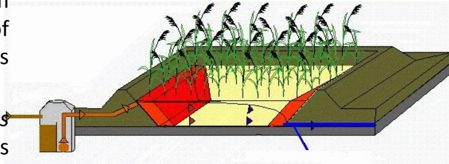
Horizontal subsurface flow (H-SSF)
