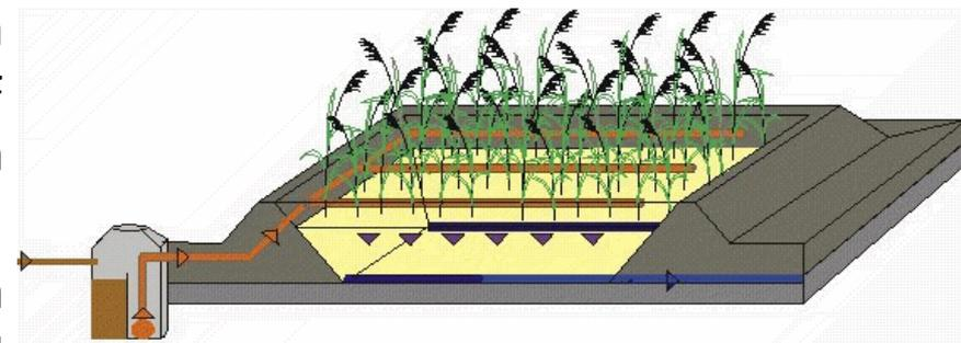
Vertical subsurface flow (V-SSF)
