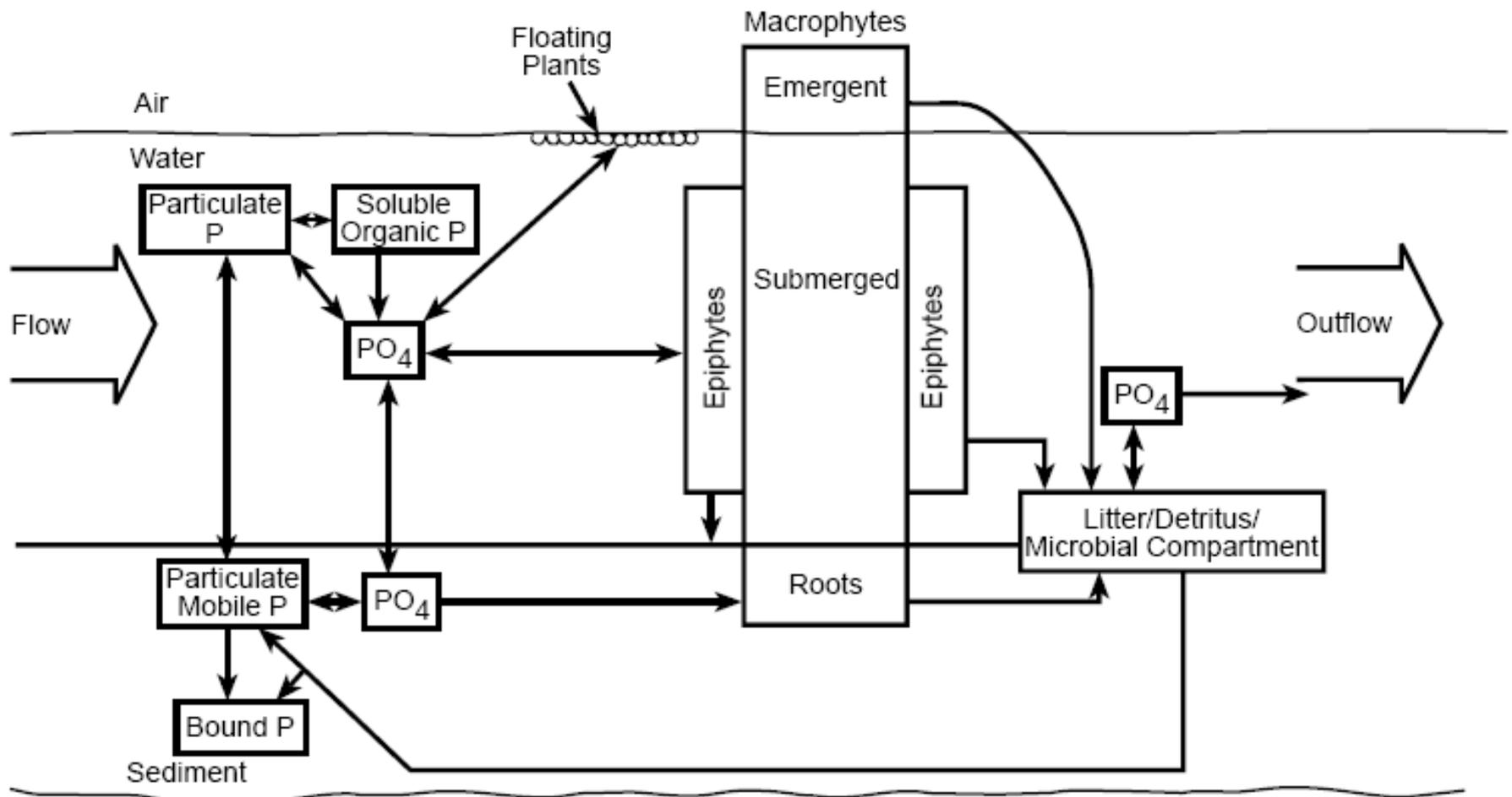
Figure 3-7. Phosphorus cycling in a FWS wetland (adapted from Twinch and Ashton, 1983)
