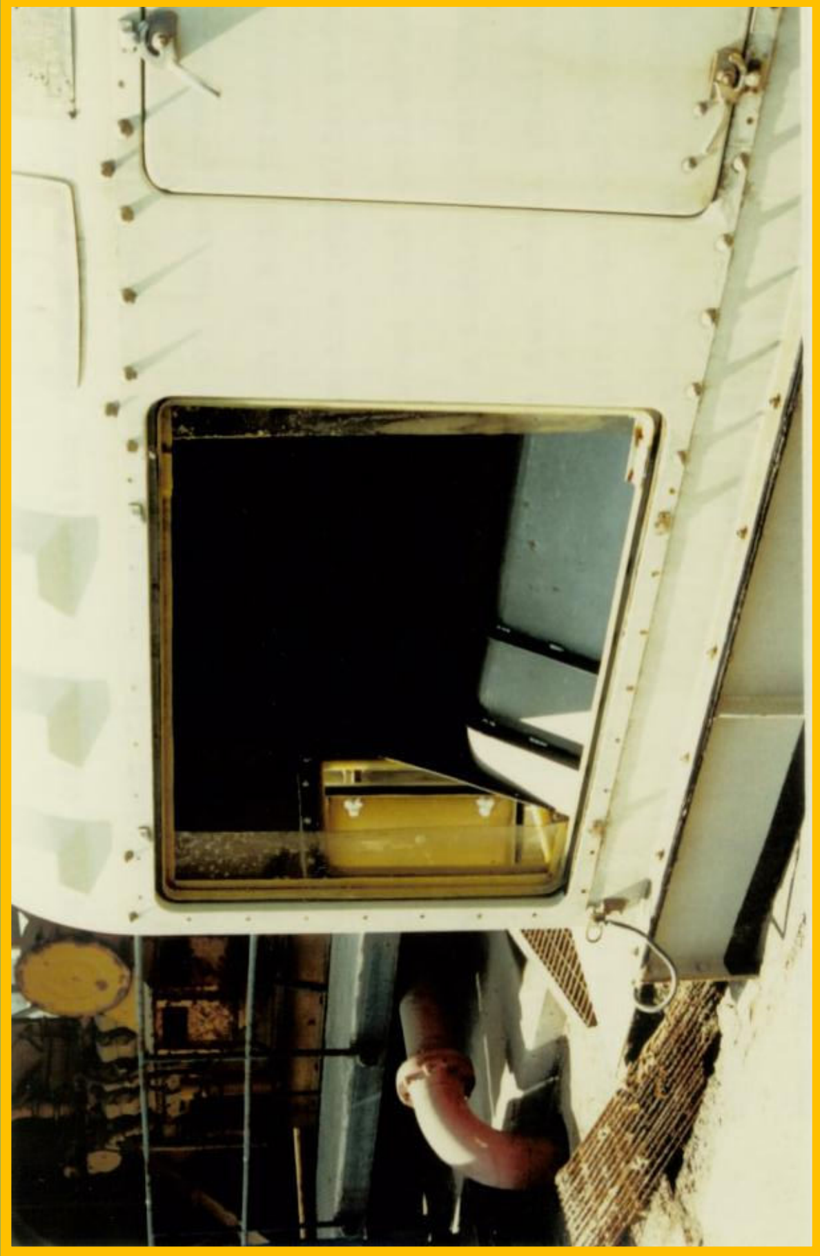
Housing of traveling screen mesh of <1\text{cm}^2
