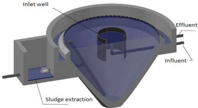
Section of a cylindrical-conical static primary settler
