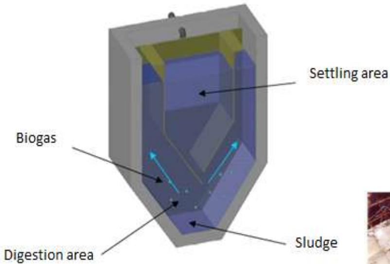
Diagram of an Imhoff tank
