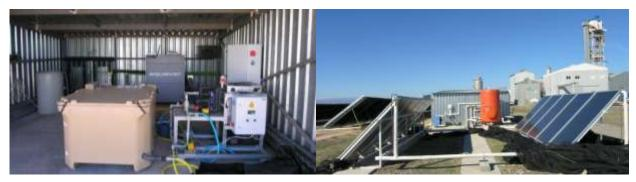
Fig. 20. Internal (left) and external (right) views of the Membrane Distillation experimental test bed within the PSA low-temperature solar thermal desalination facility
