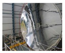
Fig. 15. Interior view of the SF-40 solar furnace, showing the parabolic concentrator
