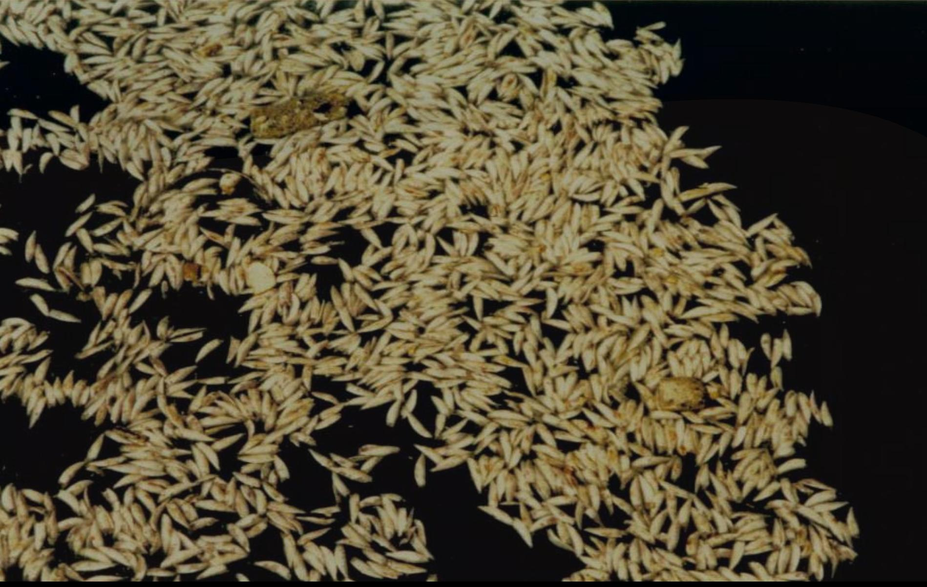
Dead Pelagic fish (Sardinella) in the forebay of desalination plant resulting from chlorination for bio-fouling control
