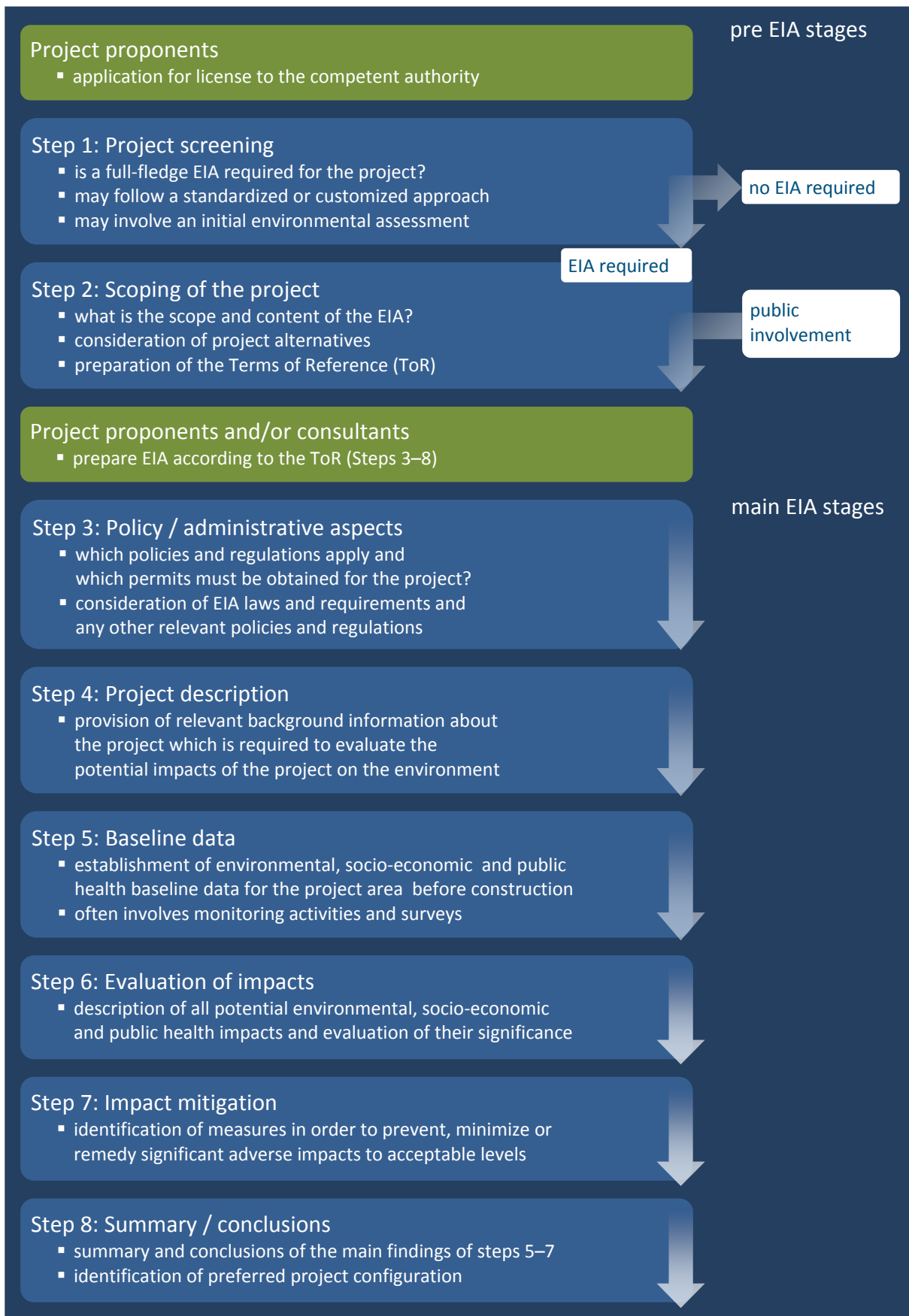
Figure 2: Pre- or early EIA phases (scoping and screening) and main EIA phase.
