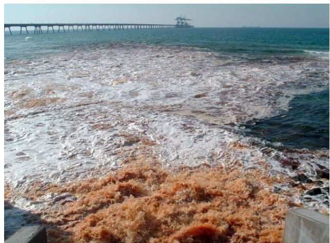
Figure 11: Periodic discharge of filter backwash water from the Ashkelon SWRO plant in Israel (courtesy of Rani Amir, Director of the Marine and Coastal Environment Division, Israel Ministry of the Environment).
