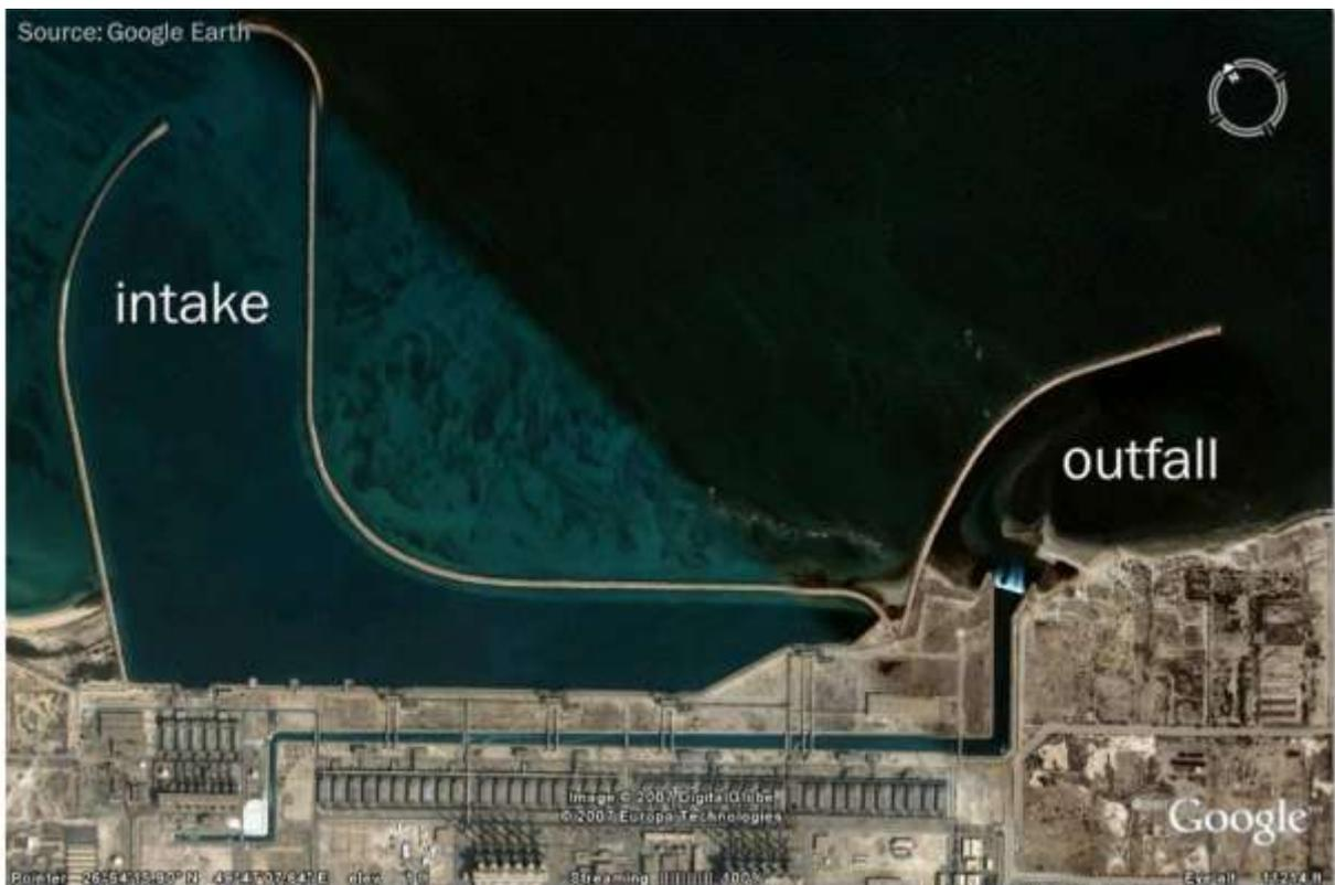
Figure 14: Al Jubail (KSA), MSF plant, Arabian Gulf, 1.54 million m<sup>3</sup>/d, positively buoyant discharge (Source: Google Earth)
