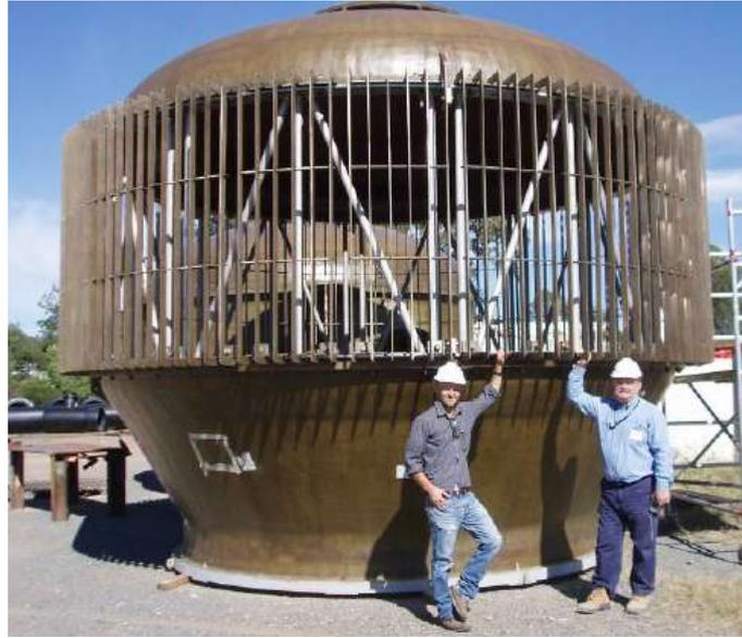
Figure 3: Open intake tower with "velocity cap". Reproduced from Cannesson et al. (2009)
