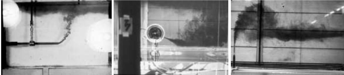
Figure 51: Pictures of laboratory experiments showing boundary interactions with the surface, the bottom and the pycnocline (courtesy of G.H. Jirka, L. Fan, Keck Lab, CIT)
