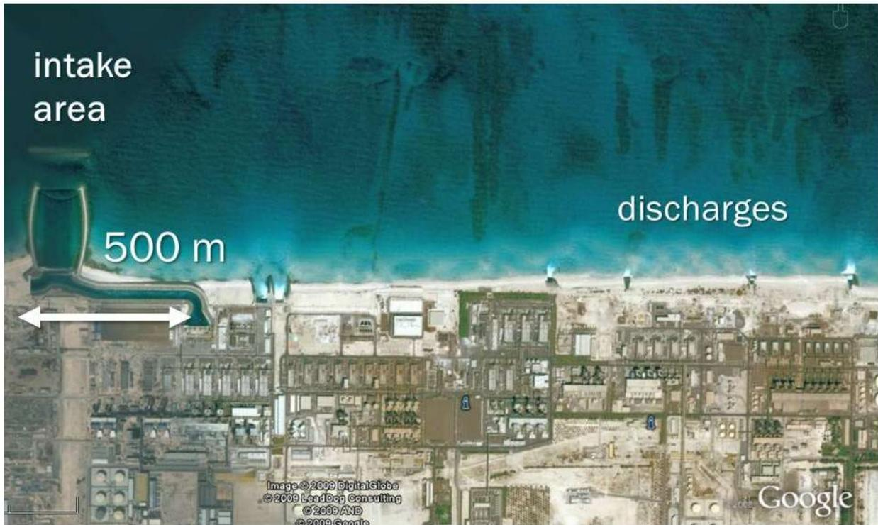
Figure 17: Jebel Ali MSF plant, UAE, power and water cogeneration plant with desalination capacity of 1.64 Mm<sup>3</sup>/d, positively buoyant discharge (Source: Google Earth)
