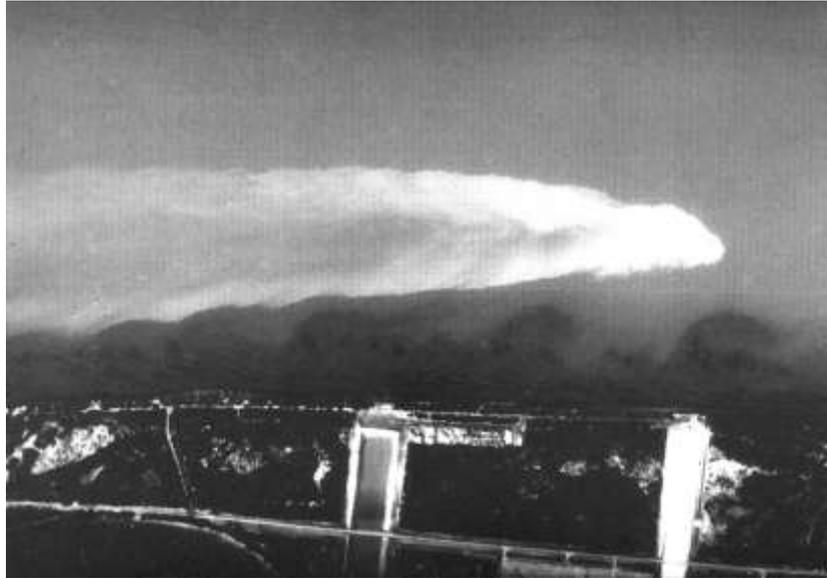
Figure 58: Surface plume in a long shore coastal current produced by a submerged sea outfall. The infrared image shows the plume produced by the cooling water discharge from a power plant at the western coast of Florida.
