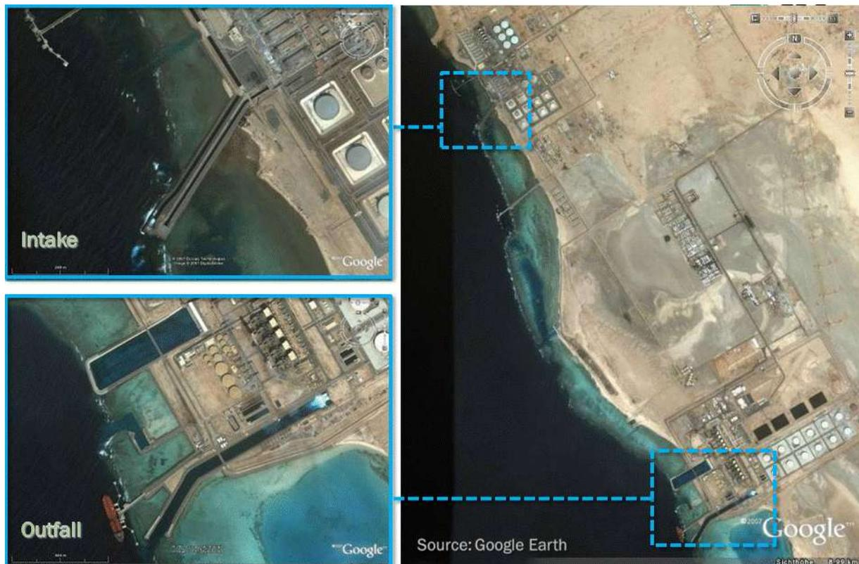
Figure 12: Shoaiba (KSA), MSF Plant, Red Sea, 1.58 million m<sup>3</sup>/d, positively buoyant discharge (Source: Google Earth)
