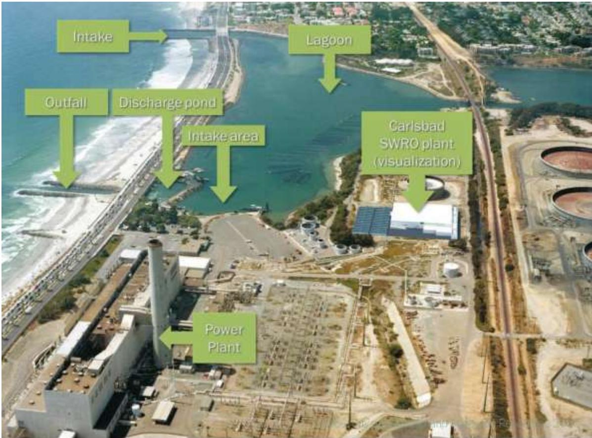
Figure 13: Carlsbad RO plant, USA, positively/negatively buoyant discharge (Source: Poseidon Resources)
