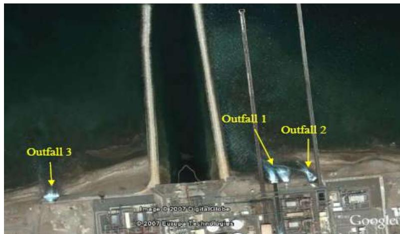
Figure 16: Al Gubrah (Oman), MSF plant, 191,000 m<sup>3</sup>/d, Gulf of Oman, positively buoyant discharge (Source: Google Earth)
