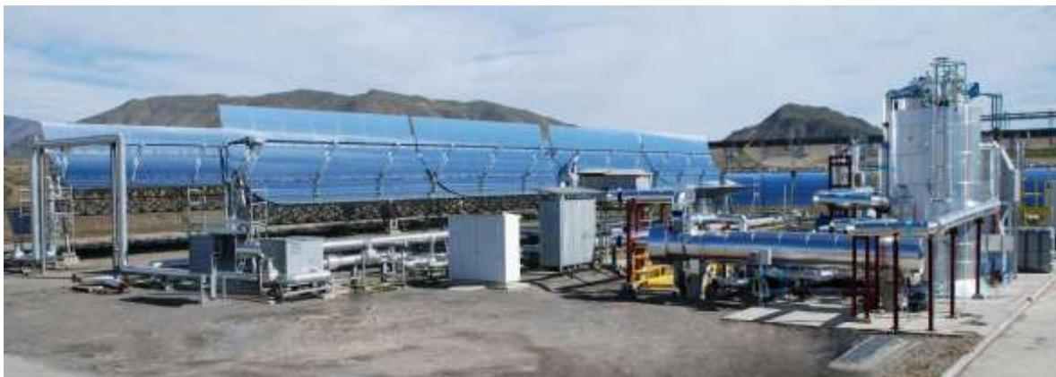
*Fig. 7. View of the pressurized gas test loop connected to a molten-salt thermal energy storage*
