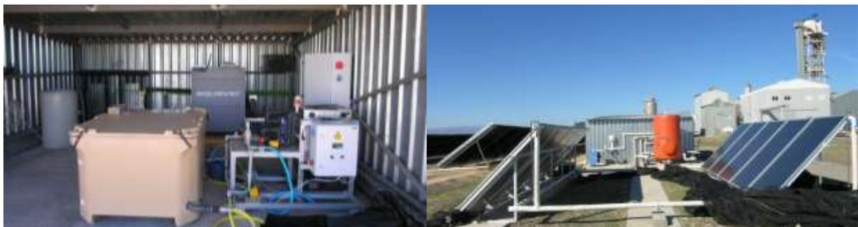
*Fig. 20. Internal (left) and external (right) views of the Membrane Distillation experimental test bed within the PSA low-temperature solar thermal desalination facility*
