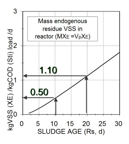
MX<sub>EH</sub> increases with sludge age (R<sub>s</sub>) but increase gets larger as sludge age gets longer due to longer duration of endogenous process.
