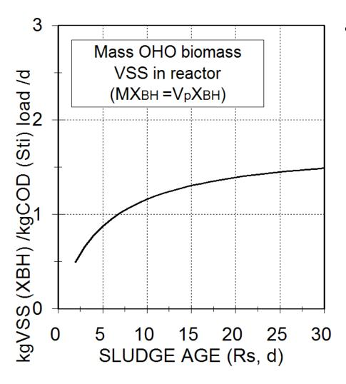
MX<sub>BH</sub> in reactor increases with sludge age (R<sub>s</sub>) but increase gets smaller as sludge age gets longer due to longer duration of endogenous process.
