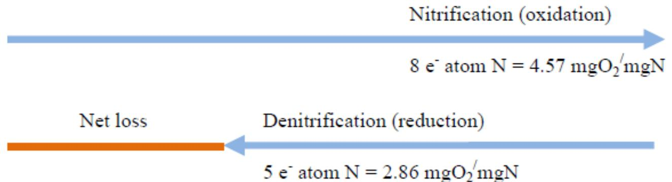
Nitrification:  $4.57 \text{ mgO}_2/\text{mgNH}_4\text{-N}$  nitrified to  $\text{NO}_3\text{-N}$
