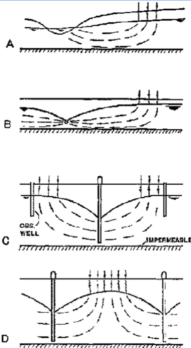
Types of Surface Spreading SAT Systems (Bouwer, 1987)
